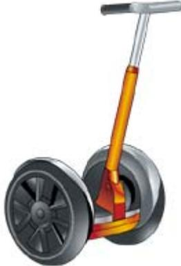
The Segway Human Transporter, also known as the Segway Personal Transporter (commonly referred to as a "Segway"), is a self-balancing, electric-powered transportation device able to turn in place and designed for one person, with a top speed of 20 km/h.
